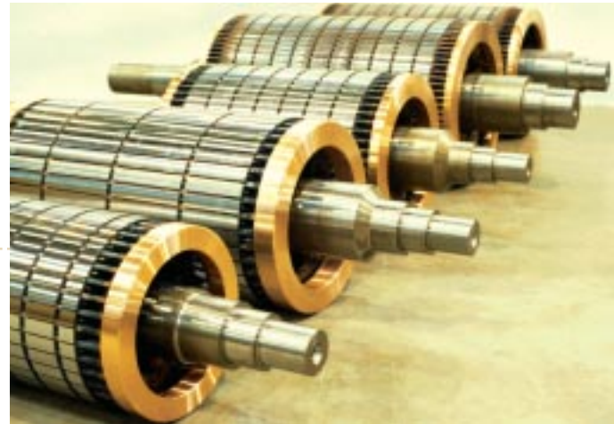
TWMC rotors are composed of copper/copper alloy.
