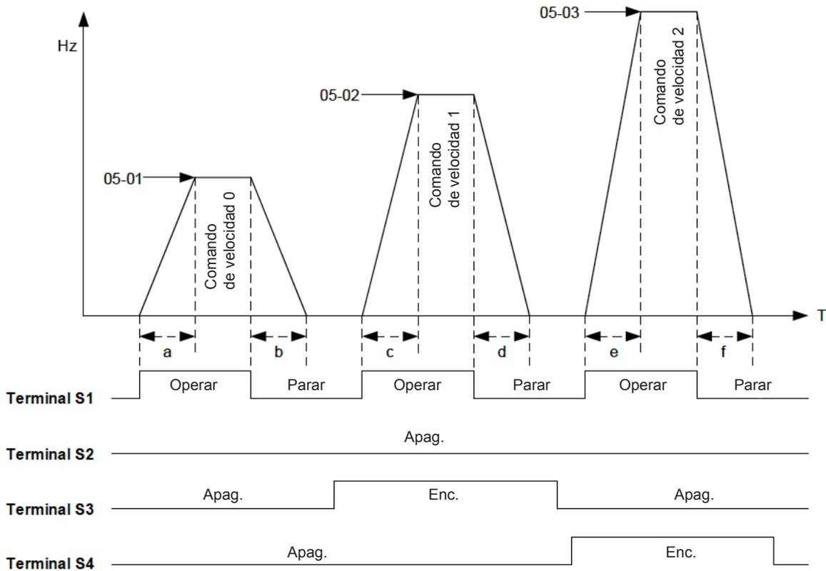
$$a = \frac{(05-17) \times (05-01)}{(01-02)} \quad b = \frac{(05-18) \times (05-01)}{(01-02)} \quad c = \frac{(05-19) \times (05-02)}{(01-02)} \quad \text{in sec.}$$
