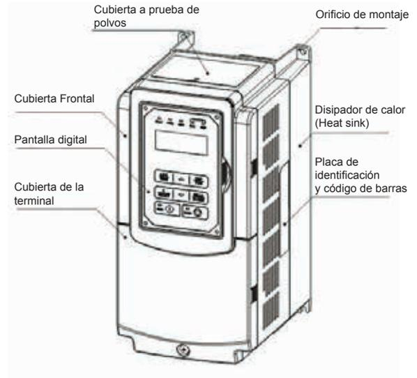
(Tipo montaje a muro, IEC IP20, NEMA 1)
