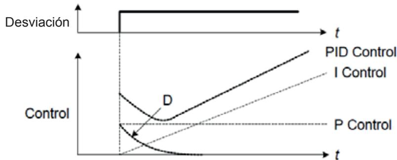
Figura 4.3.68 Control PID
