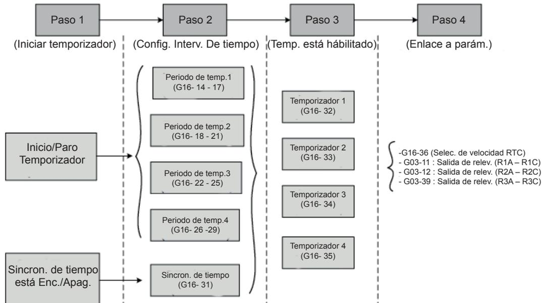
**Figura 4.3.86 Estructura RTC**
