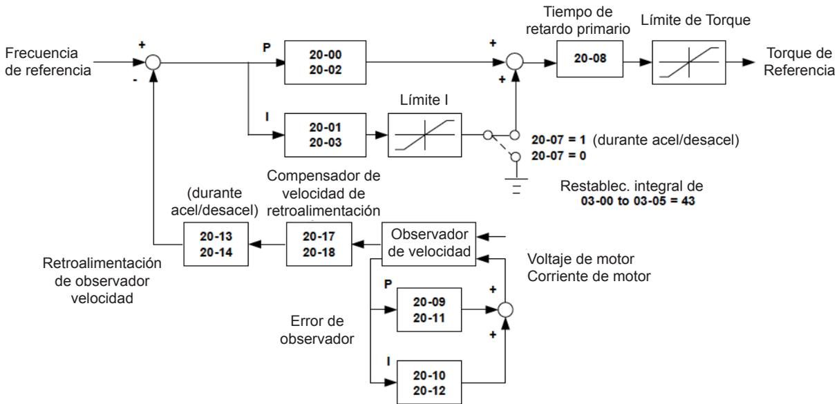
**Figura 4.3.95 Diagrama de block ASR (modo SLV)**
