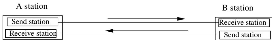
2. Half Duplex: Data is received and transmitted on one line. Both sides can't receive/send the message at the same time.
