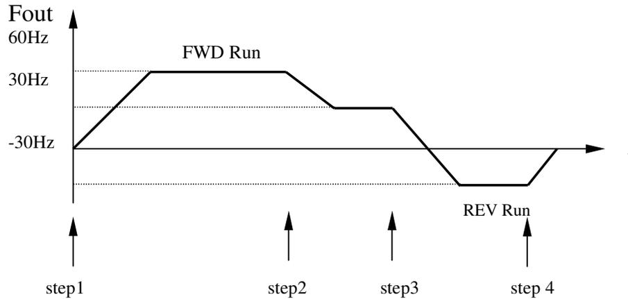
1. Let the inverter forward run by 60Hz.
