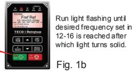
Run light flashing until desired frequency set 12-16 is reached after which light turns solid.
