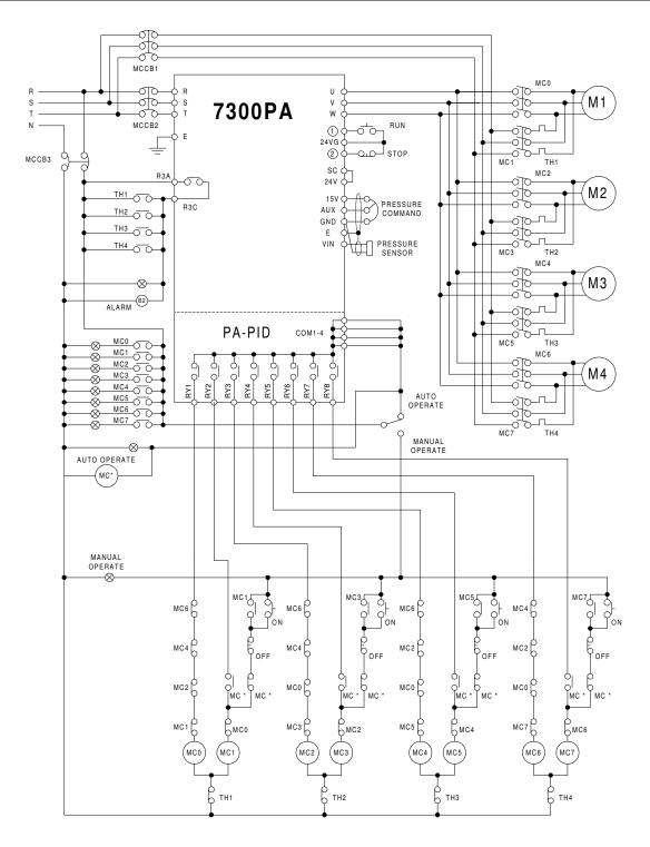
Fig 6 Fixed mode wiring diagram
