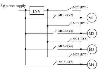
Fig 2 variable frequency pump cyclic mode.
