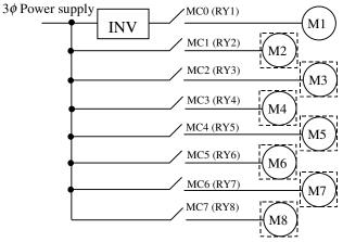
Fig 1 variable frequency pump fixed mode.
